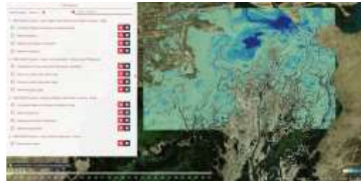
EO4SD customized product e.g. Combined Water and Wetness Probability Index for Inner Niger Delta
